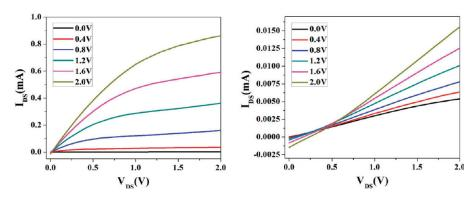
Figure 8. Output curves for SBA-ZTO (left) fresh FET and (right) FET after HMDS coating (W/L = 10).
