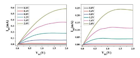
Figure 7. FET output curves after CYTOP coating, ZTO devices stored in ambient environment for 24 h (left) and 72 h (right) (W/L = 10).
