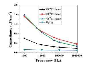
**Figure 5.** Frequency-dependent capacitance measurements for 90 nm  $Al_2O_3$  and 80 nm SBA thin films annealed at different temperatures.
