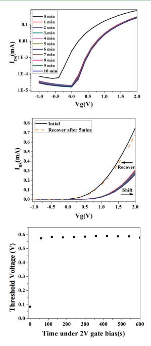
**Figure 9.** (top) Transfer curve of the ZTO/SBA under gate bias 2 V (W/L = 10). (middle) Transfer curve recovery after 5 min. (bottom) Threshold voltage shift under gate bias without Cytop coating.
