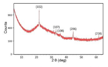
Figure 4. XRD pattern for SBA 90 nm spin coated thin film after annealing at 1000  $^\circ$ C for 15 h.
