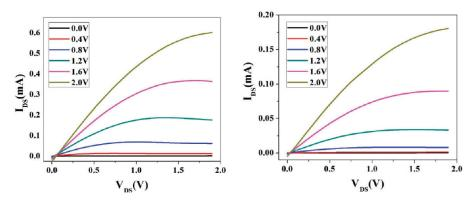
Figure 6. Output curves for (left) fresh ZTO FET and (right) ZTO FET stored in ambient environment for 24 h (W/L ratio = 10).
