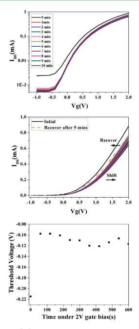
**Figure 10.** (top) Transfer curve of the ZTO/SBA after coating with Cytop under gate bias 2 V. (middle) Transfer curve recovery after 5 min (W/L = 10). (bottom) Threshold voltage shift under gate bias with Cytop coating.
