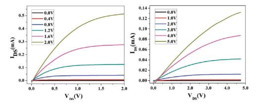
Figure 1. Comparison of output curve of ZTO/SBA (left) and ZTO/Al<sub>2</sub>O<sub>3</sub> (right) devices (80 nm SBA, 90 nm Al<sub>2</sub>O<sub>3</sub>, and W/L ratio = 10). Insets show gate voltages.
