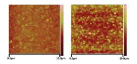
**Figure 2.** AFM picture of SBA (left) and  $Al_2O_3$  (right) gate layer. The squared-off feature edges are an artifact of the scanning direction.
